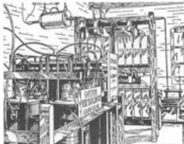
Fig. 1. A drawing of the Poldhu 1901 spark transmitter, after a contemporary photograph [see footnote 29 below]; note the spark gap by the window which is retouched in the photograph. The inductors are in the foreground (e.g., H12), and the condensers towards the back, with horizontal handles on their drawers.
